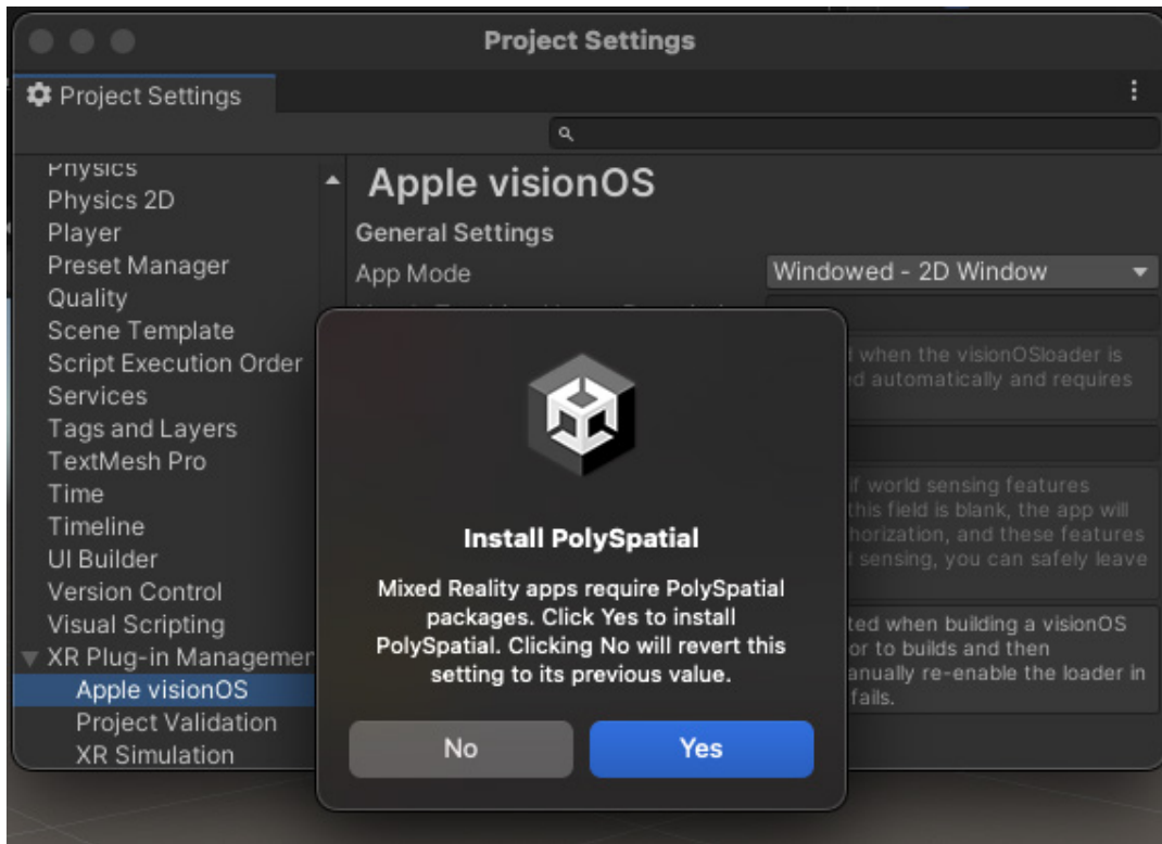
Both the visionOS Plugin and Polyspatial packages are required for creating MR apps
